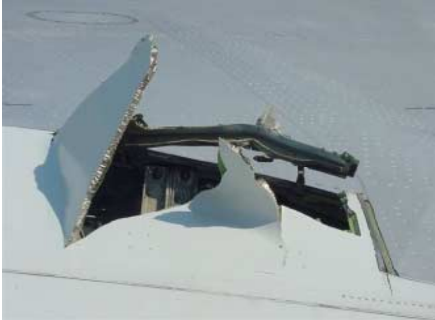
Figure 4 –Damage on the Upper Wing Caused by Exiting Debris
