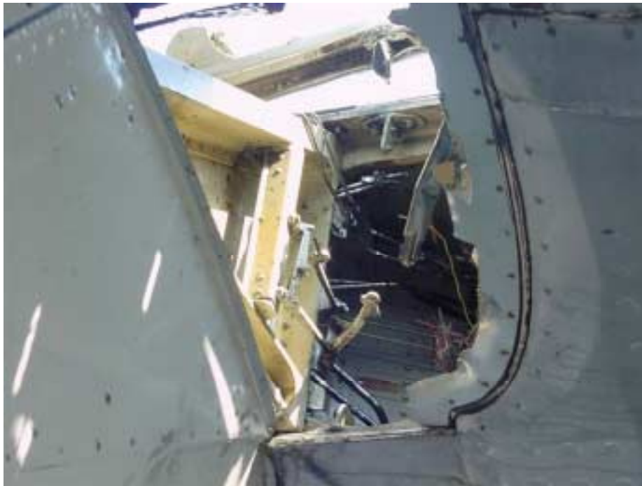
Figure 3 – Damage to the Lower Wing Access Panel (view from below)
