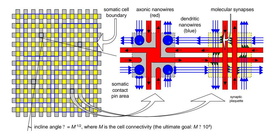
This architecture allows to combine high density CMOS-based somatic cells (up to 10<sup>8</sup> per cm<sup>2</sup>) with extremely high density of single-electron latching switches working as synapses (up to 10<sup>12</sup> per cm<sup>2</sup>) necessary for our "final" goal: placing a hardware analog of a mammal cerebral cortex on a 10?10 cm<sup>2</sup> silicon area. K. Likharev, SUNY Stony Brook
