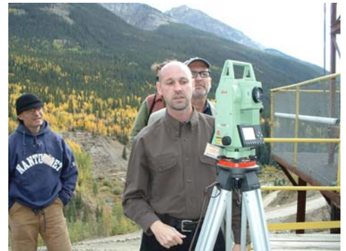
NPS HAER Architect Dana Lockett, demonstrating the Lieca total station survey equipment used document historic structures at the mill site. This digitally mapped information is downloaded in to Auto Cad software to create measured drawings. Mr. Lockett gave a seminar presentation explaining this process and the HAER standards associated with the production of these drawings in a morning lecture venue.
