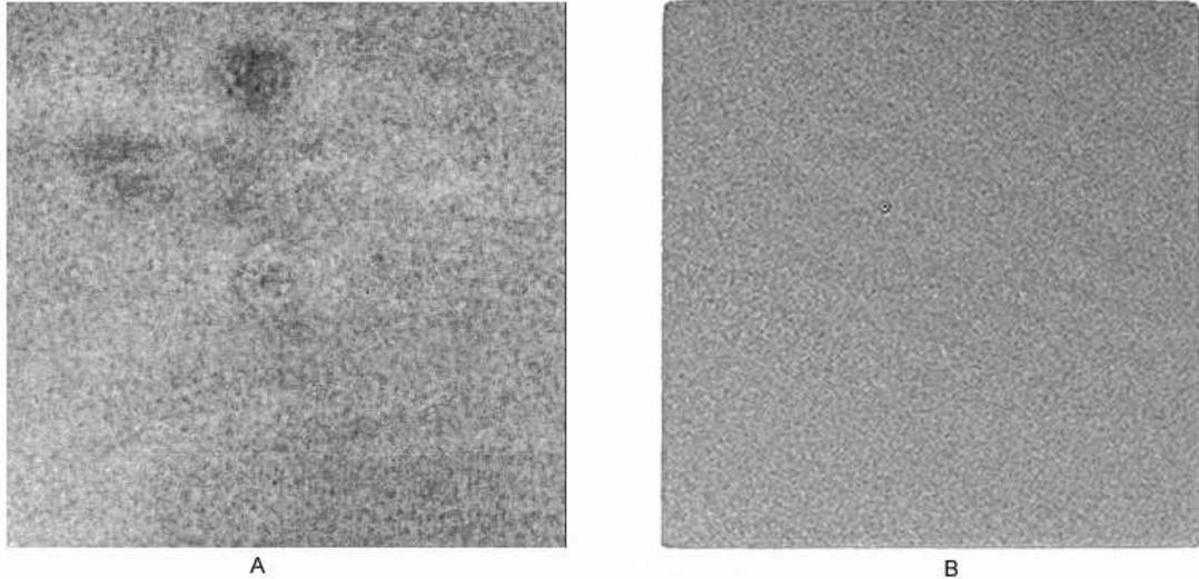
**Figure 7.** Acoustic images: (A) an 18K gold coupon and (B) a 22K gold coupon
