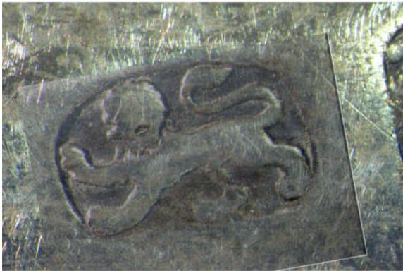
**Figure 9.** A recovered acoustic image of a worn-off lion hallmark overlaying a digital image of an identical hallmark from the same set of teaspoons.
