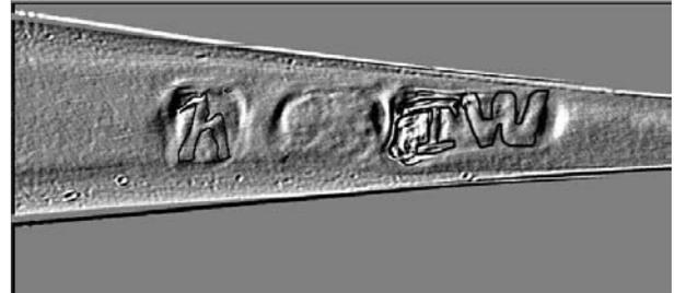
**Figure 20.** Image processed acoustic image with the date letter “h” and the maker’s initials “TW” outlined for clarity. The third hallmark is still illegible but resembles the lion passant mark for sterling quality metal.
