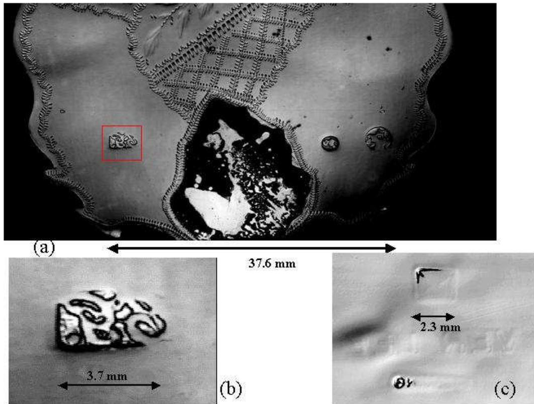
**Figure 11.** Ultrasonic back-wall image of the sterling silver blade of a French fish knife dated approximately 1875 to 1925. One hallmark is isolated (b) and magnified for comparison to the back-wall image of the coupon (c). No deformation appears to extend from the fish knife hallmark.
