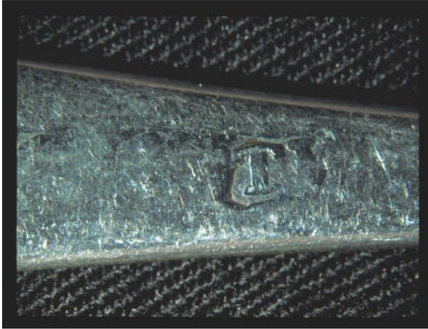
**Figure 18.** Photograph of a teaspoon with one partially readable hallmark and two illegible hallmarks.
