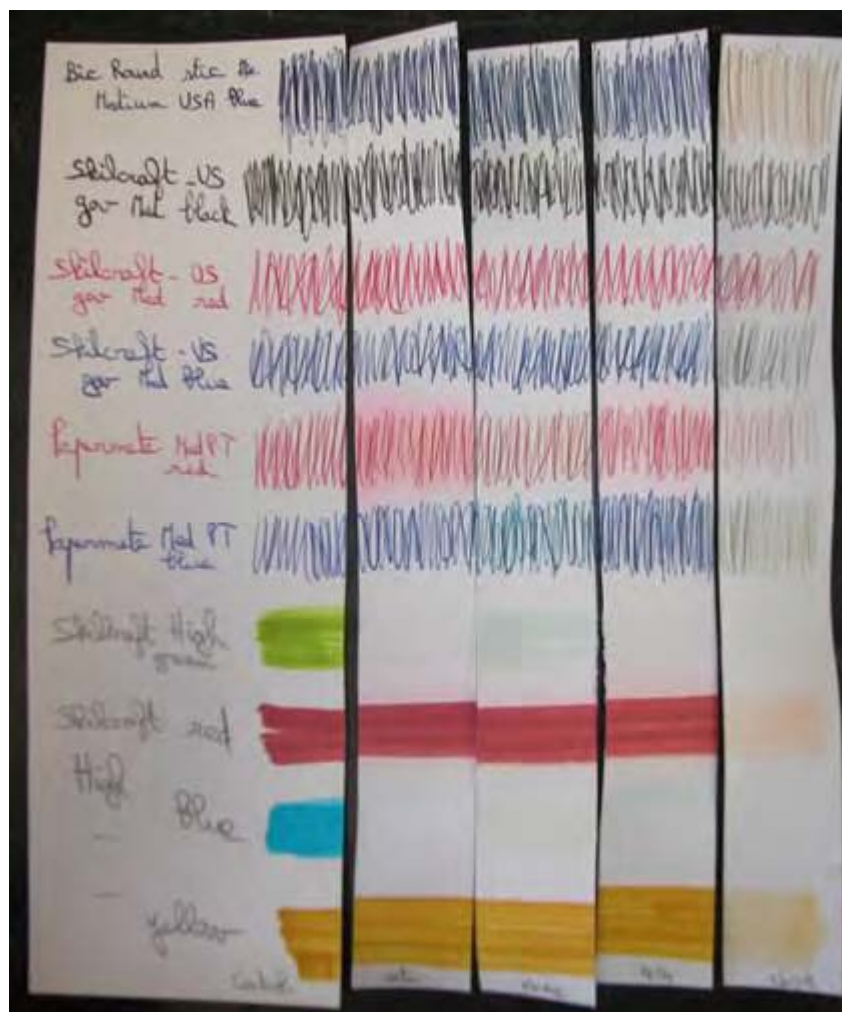
Figure 3: samples of writing inks treated by immersion for 30 minutes in water, H_2O_2 , Oxone ® and NaOCl.
