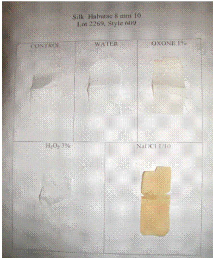
Figure 6: silk samples treated by immersion for 30 minutes in water, H 2 O 2 , Oxone ® and NaOCl.
