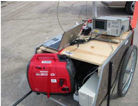
Figure 3: Mobile receiving cart.
