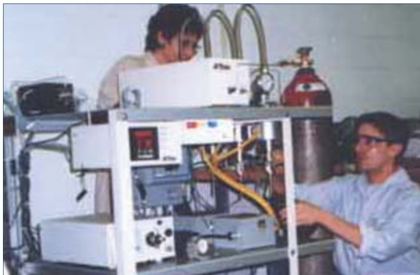
Two employees of Thar Technologies check one of the company's supercritical fluid systems.
