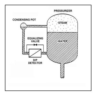
Refer to the drawing of a differential pressure (D/P) level detection system for a pressurizer at normal operating temperature and pressure (see figure below).
