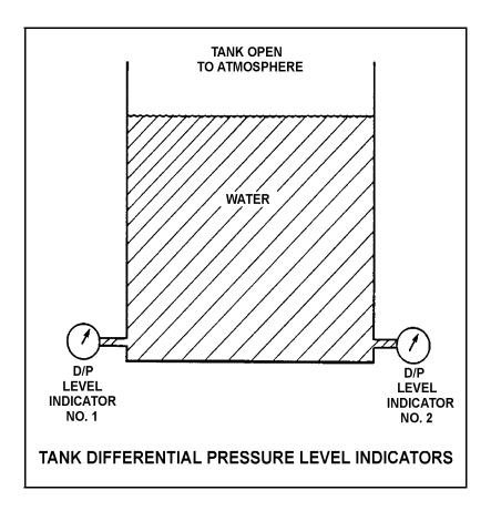
Refer to the drawing of a water storage tank with two differential pressure (D/P) level indicators (see figure below).
