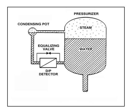
Refer to the drawing of a tank differential pressure level detector that was recently calibrated at a tank water temperature of  $80^{\circ}$ F (see figure below).
