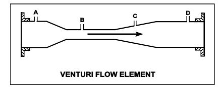
A cooling water system is operating at a steady-state flow rate of 500 gpm with 60 psid across the flow transmitter venturi. If cooling water flow rate is increased to 1000 gpm, differential pressure across the flow transmitter venturi will be approximately...
