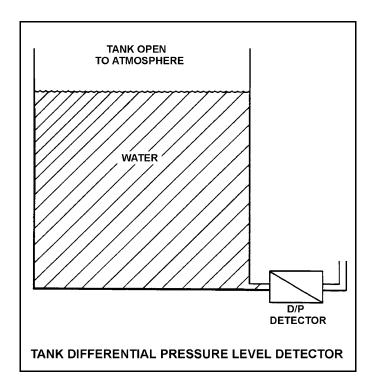
Refer to the drawing of two tank differential pressure (D/P) level indicators (see figure below).
