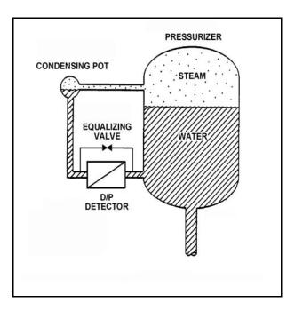
Refer to the drawing of a differential pressure (D/P) level detection system for a pressurizer at normal operating temperature and pressure (see figure below).
