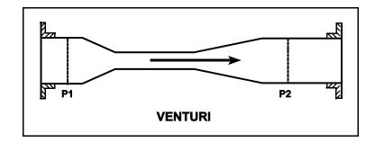
Subcooled water is flowing through a venturi flow element. When the water reaches the throat of the venturi, the \_\_\_\_\_\_ water pressure and the \_\_\_\_\_\_ water velocity occurs.
