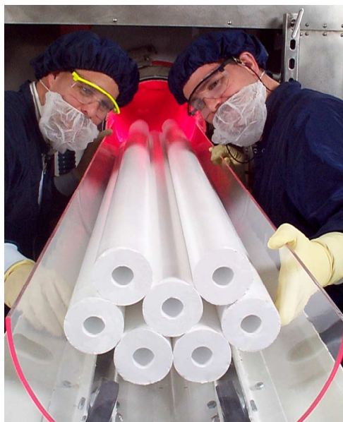
Figure 5.1. Photo of sol-gel preforms. The dried, unconsolidated tubes are being loaded into a silica “boat” to be heated in various gases to remove organic compounds, water, and refractory impurities (courtesy Bell Labs/Lucent Technologies).
