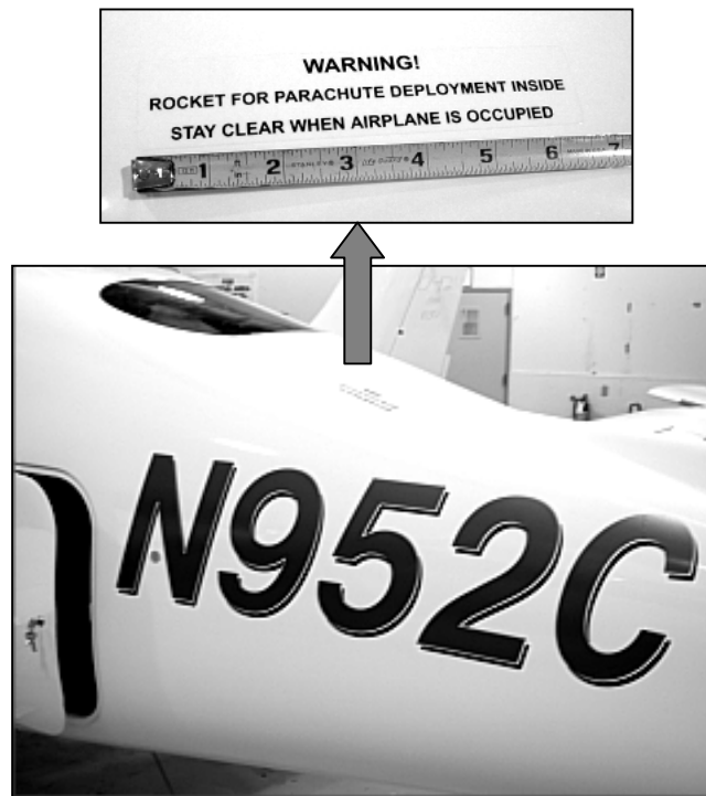
Figure 1. CAPS warning label for Cirrus SR20 and SR22 airplanes
