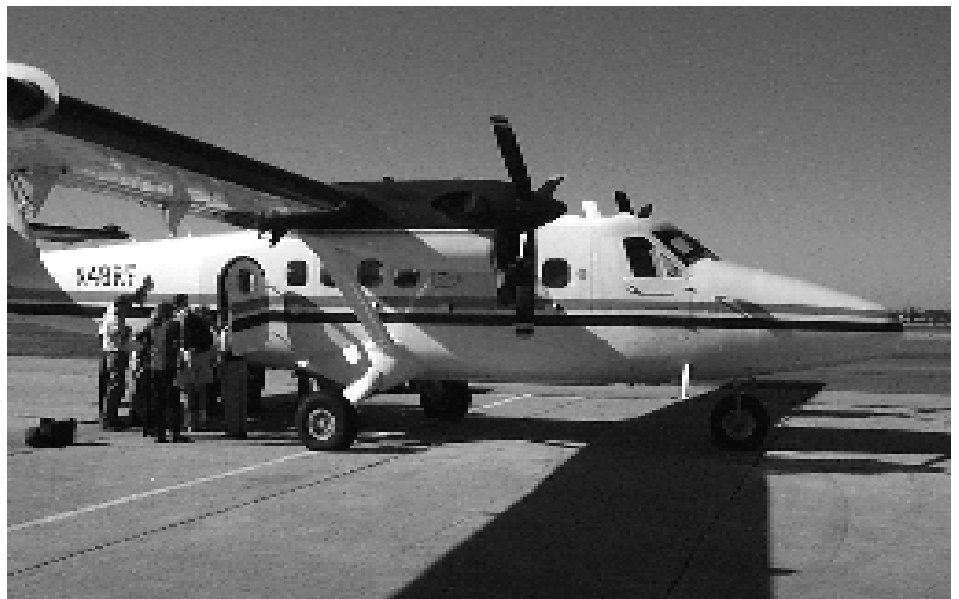
▲ Figure 1. The NOAA Twin Otter, equipped with the Airborne Topographic Mapper, is used for laser beach mapping.
