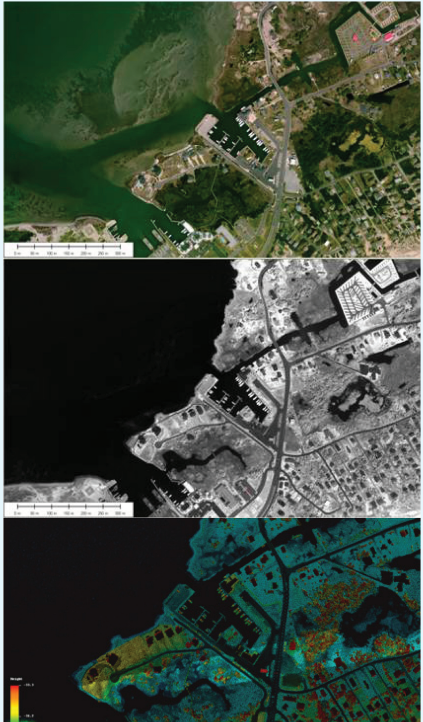
▲ Examples of data products being supplied through the NOAA-North Carolina IOCM project: color orthophoto (top), near infrared orthophoto suitable for shoreline delineation (middle), and lidar point cloud data color-coded by elevation (bottom).
