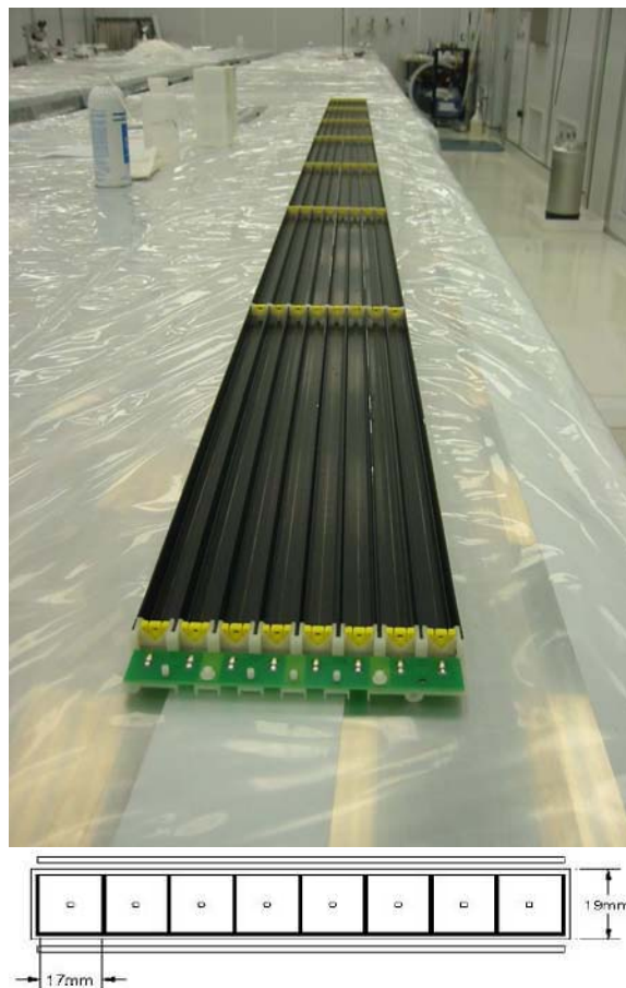
Figure 3.22: The mechanical structure of BABAR LSTs.
