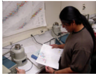
Student Conrad Valencia working with the Chart of Nuclides and a Geiger-Mueller detector to identify beta radiation energy.
