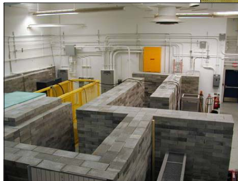
Test cell occupying a 13 m x 11 m area includes a cave shield with a borated polyethylene shield (blue plate, far left) and guard structure (yellow) for the shield door, surrounded by labyrinth of stacked concrete blocks, 0.6m thick and 2.44 m tall.
