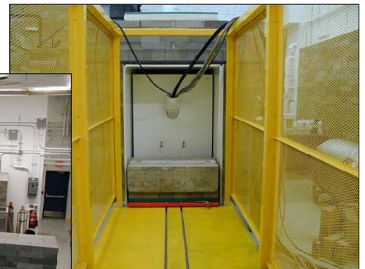
Cave shield and the 3-ton door with the (D-T) head mounted and placed on four air bearings and floor guarding.
