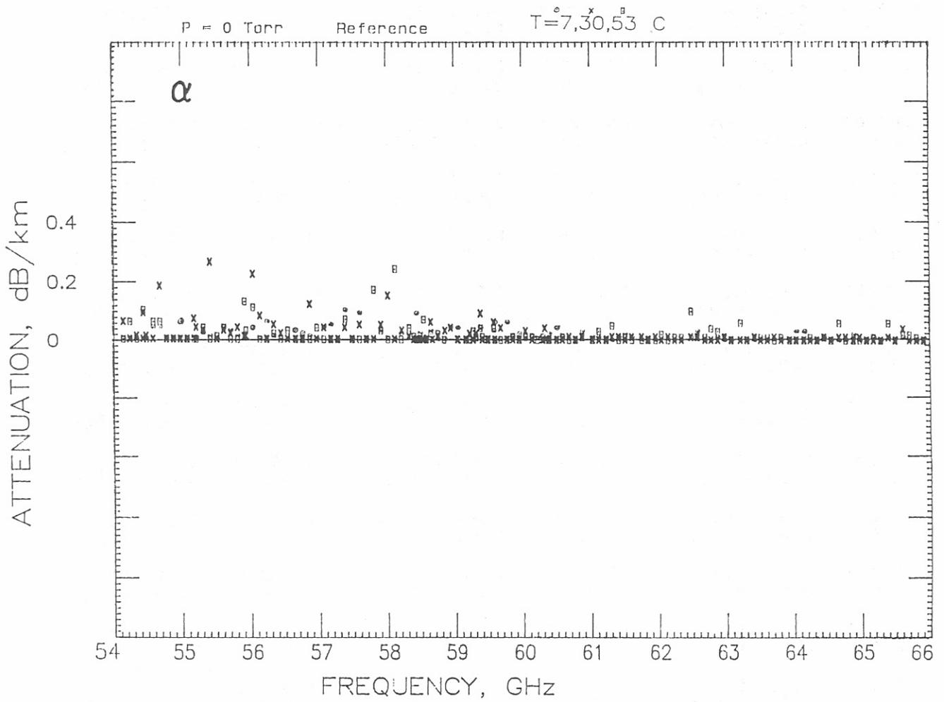
Figure A-12a. Predicted and measured attenuation rates of dry air,  $\alpha_M$  and  $\alpha_x$ , at P = 0 kPa (see RE) for frequencies between 54 and 66 GHz.
