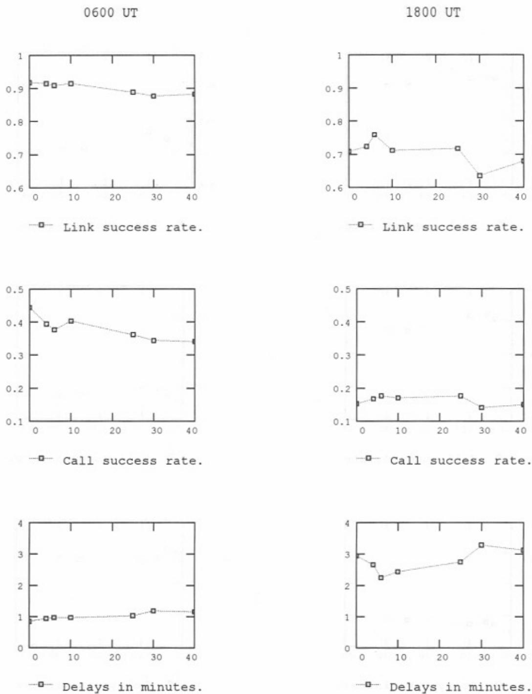
Figure E-17. Simulated network performance for 0600 and 1800 (UT) - 0, 4, 6, 10, 15, 30, and 40 scheduled sounds per hour - propagation condition 8 - 15 messages per hour.
