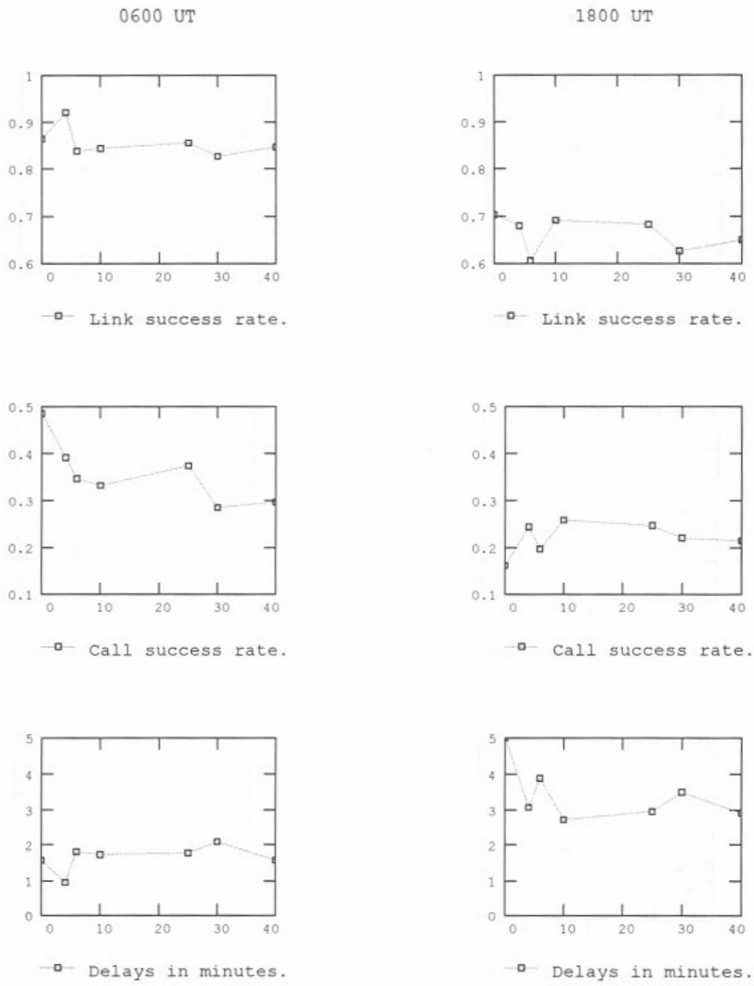
Figure E-11. Simulated network performance for 0600 and 1800 (UT) - 0, 4, 6, 10, 15, 30, and 40 scheduled sounds per hour - propagation condition 5 - 5 messages per hour.
