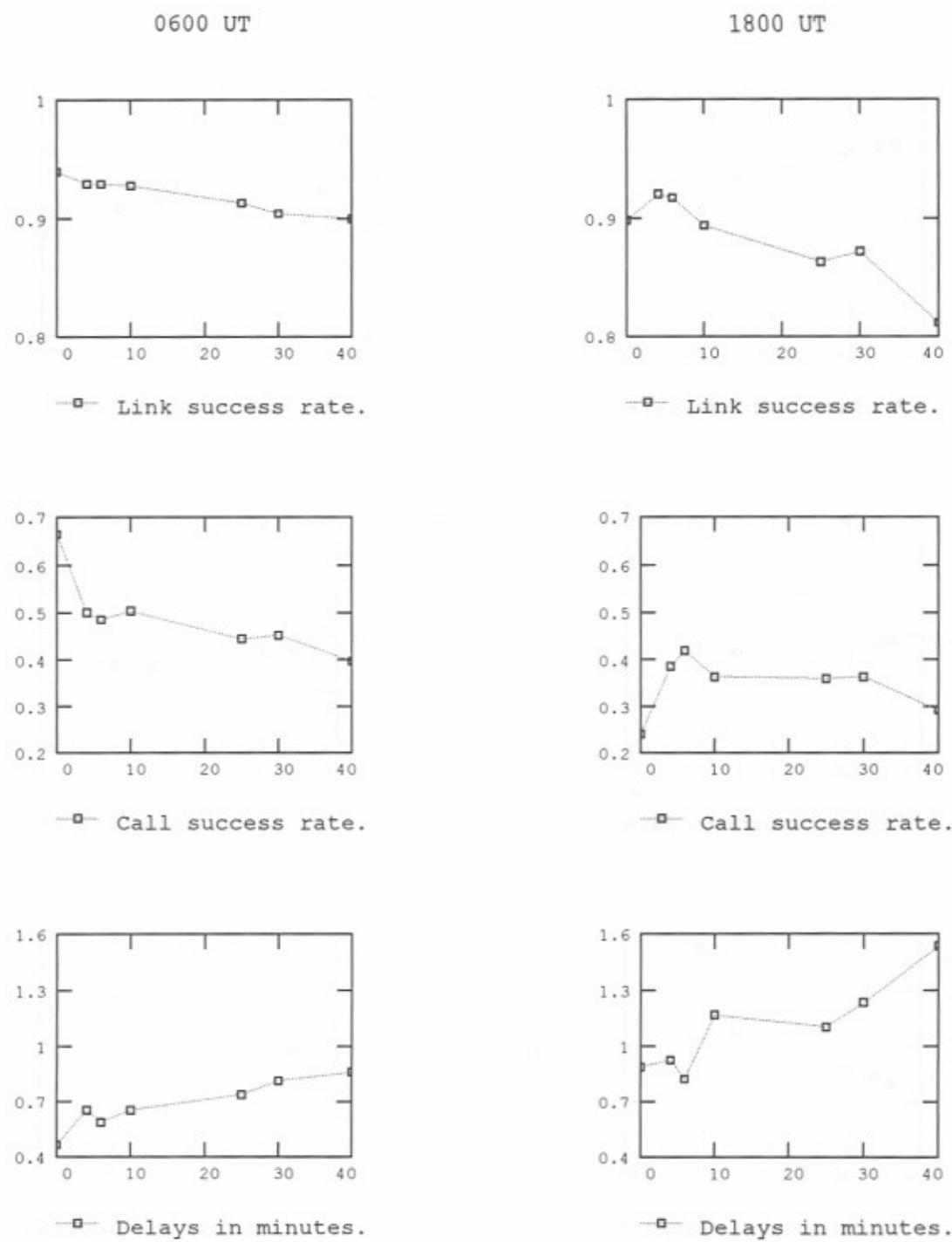
Figure E-7. Simulated network performance for 0600 and 1800 (UT) - 0, 4, 6, 10, 15, 30, and 40 scheduled sounds per hour - propagation condition 3 - 10 messages per hour.
