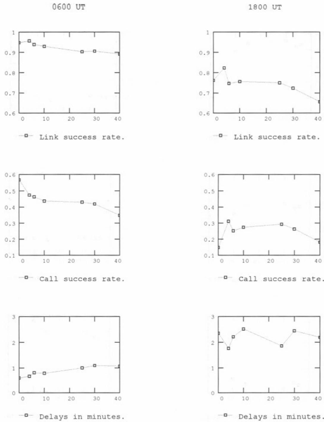
Figure E-15. Simulated network performance for 0600 and 1800 (UT) - 0, 4, 6, 10, 15, 30, and 40 scheduled sounds per hour - propagation condition 8 - 5 messages per hour.
