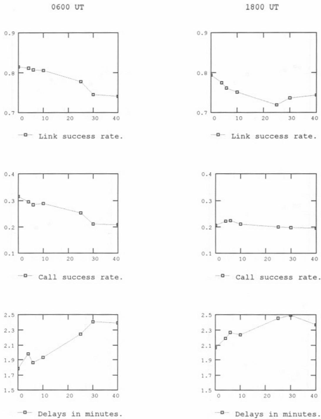
Figure E-9. Simulated network performance for 0600 and 1800 (UT) - 0, 4, 6, 10, 15, 30, and 40 scheduled sounds per hour - propagation condition 3 - 30 messages per hour.
