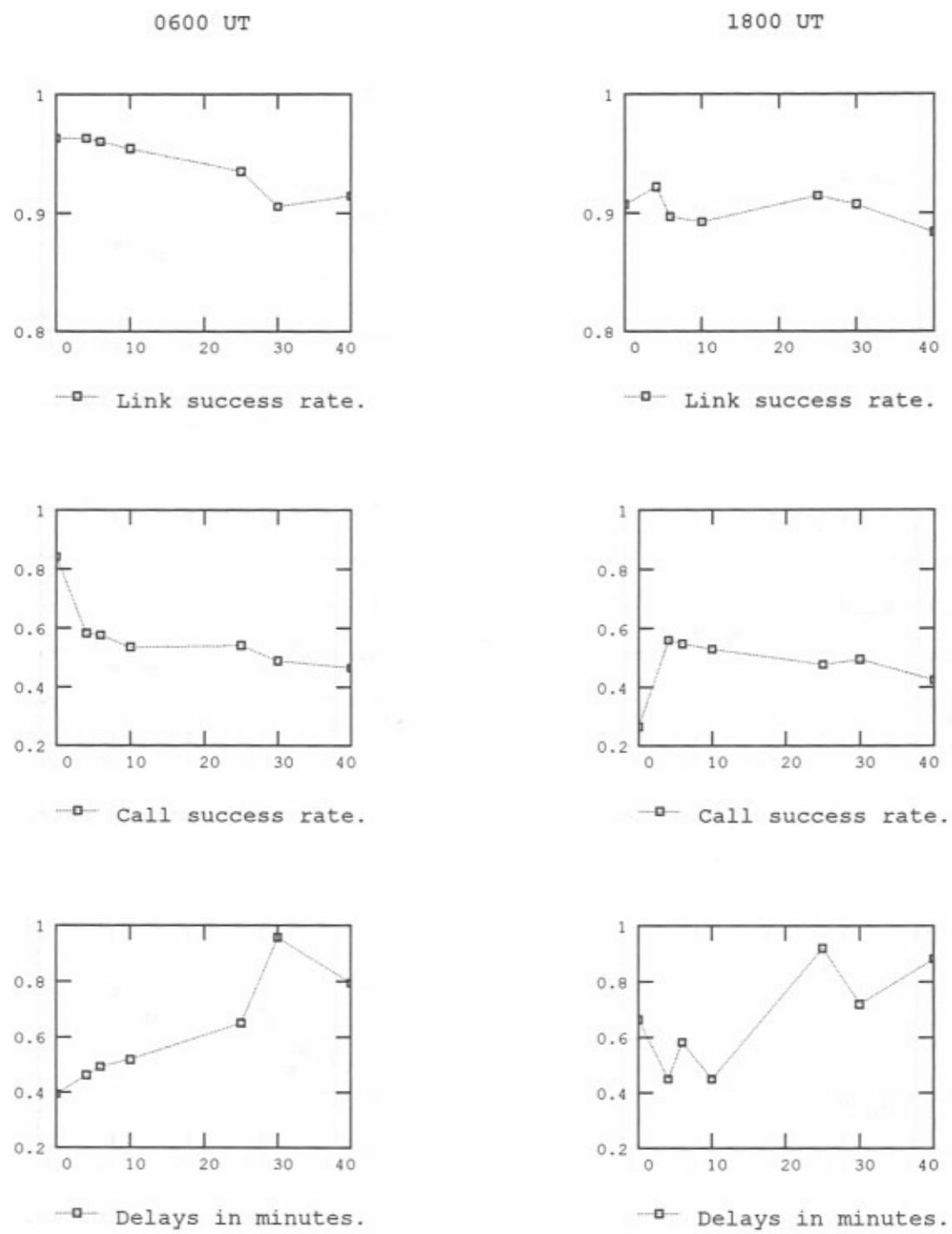
Figure E-6. Simulated network performance for 0600 and 1800 (UT) - 0, 4, 6, 10, 15, 30, and 40 scheduled sounds per hour - propagation condition 3 - 5 messages per hour.
