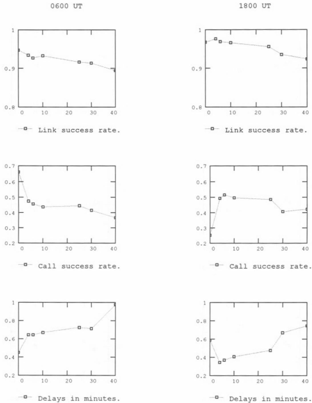
Figure E-2. Simulated network performance for 0600 and 1800 (UT) - 0, 4, 6, 10, 15, 30, and 40 scheduled sounds per hour - propagation condition 1 - 10 messages per hour.
