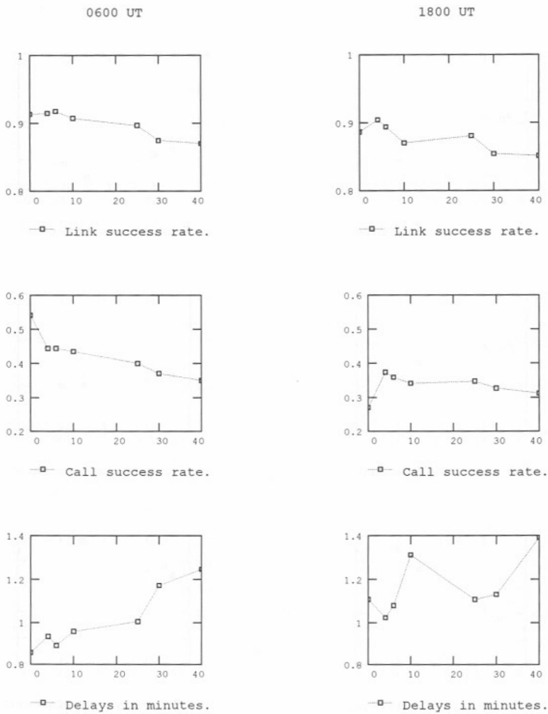
Figure E-8. Simulated network performance for 0600 and 1800 (UT) - 0, 4, 6, 10, 15, 30, and 40 scheduled sounds per hour - propagation condition 3 - 15 messages per hour.
