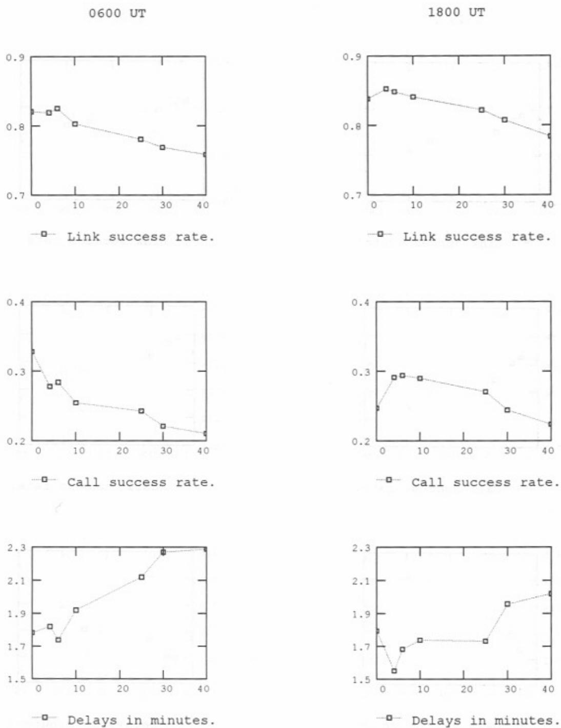
Figure E-4. Simulated network performance for 0600 and 1800 (UT) - 0, 4, 6, 10, 15, 30, and 40 scheduled sounds per hour - propagation condition 1 - 30 messages per hour.
