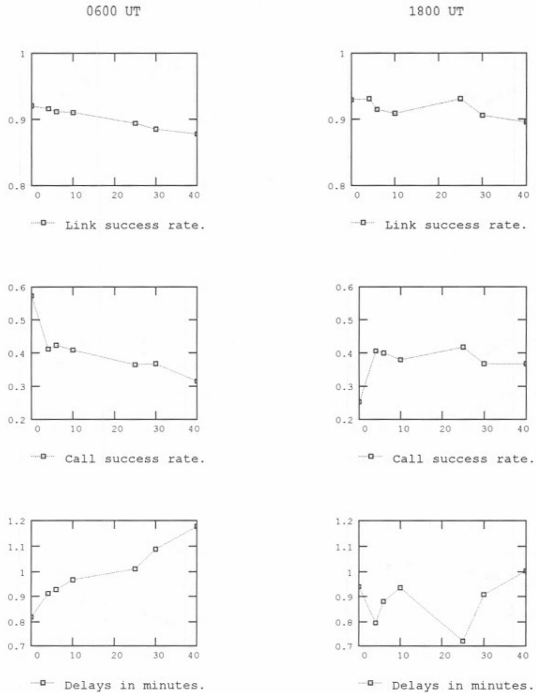
Figure E-3. Simulated network performance for 0600 and 1800 (UT) - 0, 4, 6, 10, 15, 30, and 40 scheduled sounds per hour - propagation condition 1 - 15 messages per hour.
