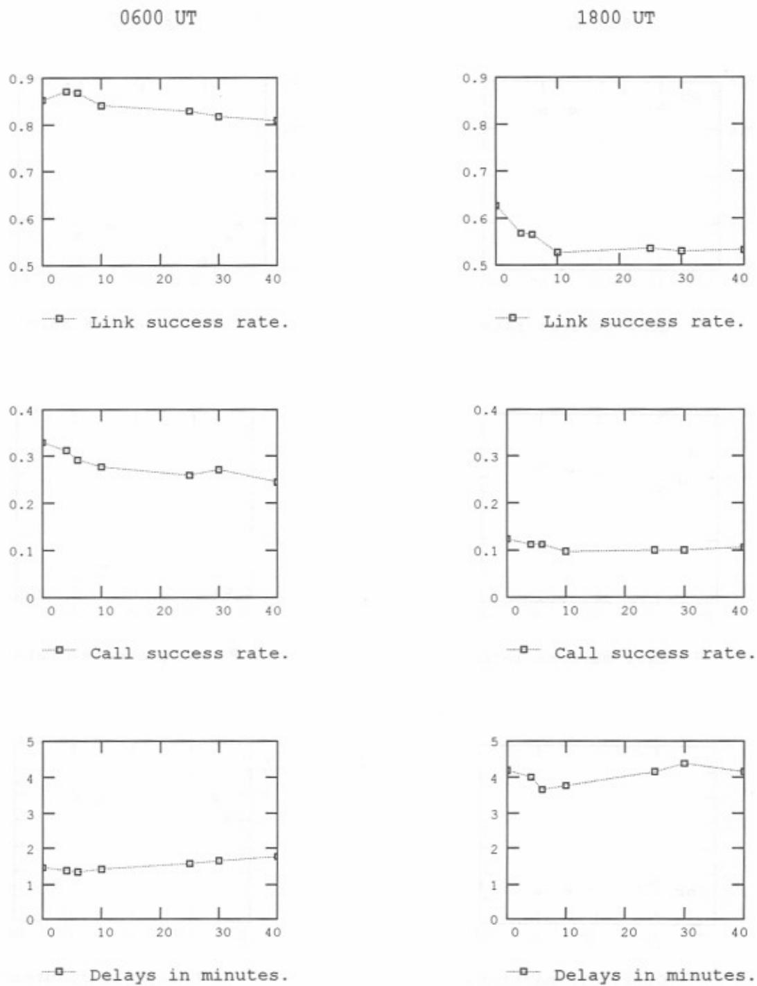
Figure E-13. Simulated network performance for 0600 and 1800 (UT) - 0, 4, 6, 10, 15, 30, and 40 scheduled sounds per hour - propagation condition 5 - 15 messages per hour.
