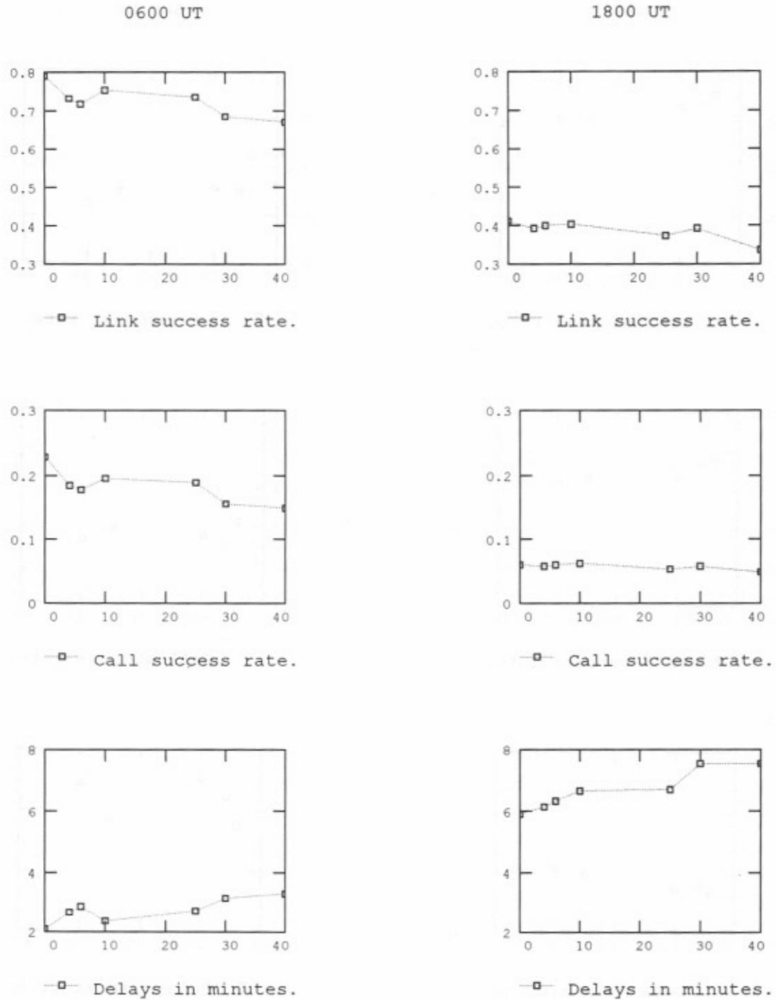
Figure E-14. Simulated network performance for 0600 and 1800 (UT) - 0, 4, 6, 10, 15, 30, and 40 scheduled sounds per hour - propagation condition 5 - 30 messages per hour.
