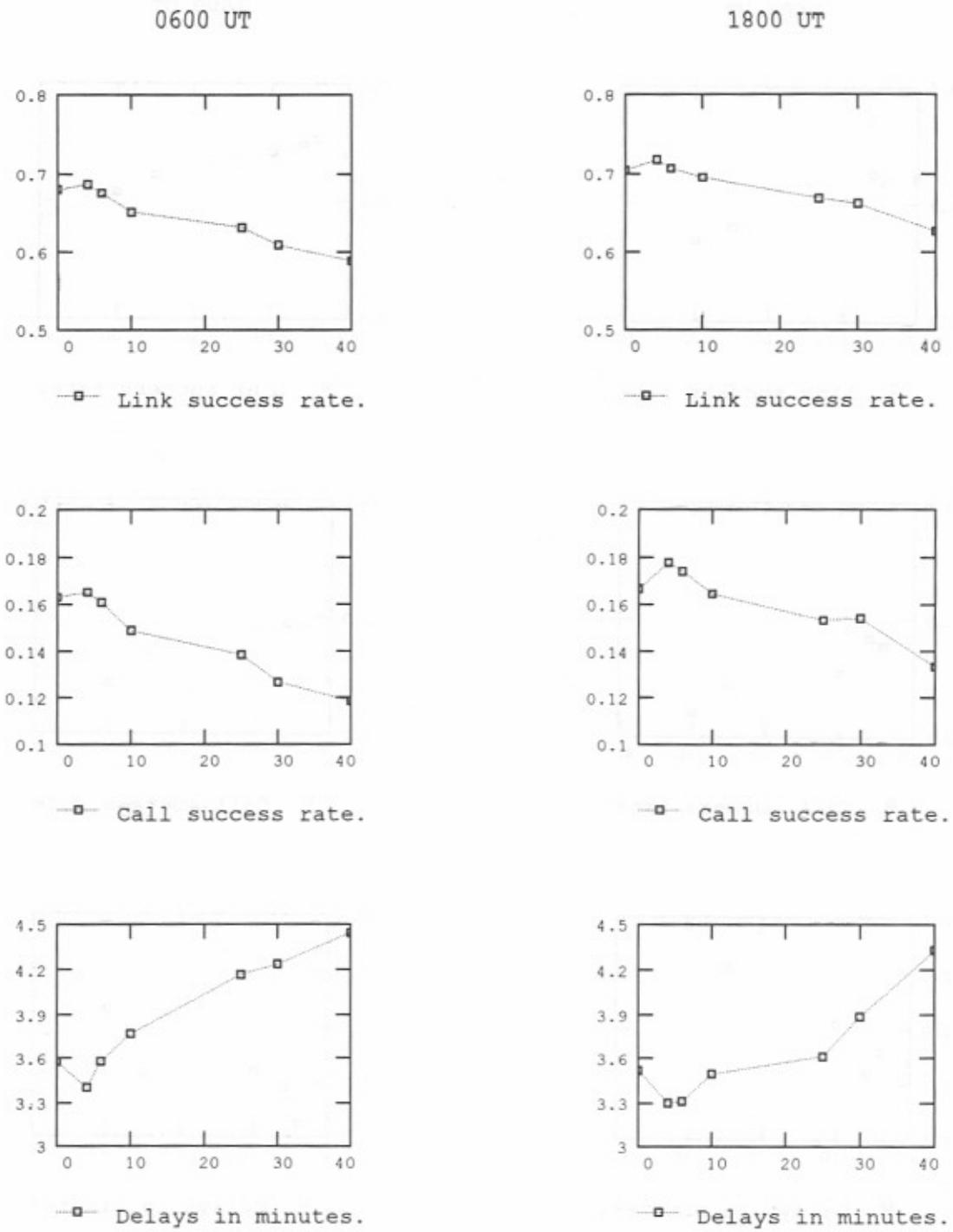
Figure E-5. Simulated network performance for 0600 and 1800 (UT) - 0, 4, 6, 10, 15, 30, and 40 scheduled sounds per hour - propagation condition 1 - 45 messages per hour.
