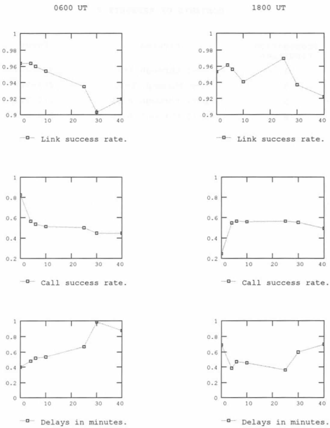
Figure E-1. Simulated network performance for 0600 and 1800 (UT) - 0, 4, 6, 10, 15, 30, and 40 scheduled sounds per hour - propagation condition 1 - 5 messages per hour.
