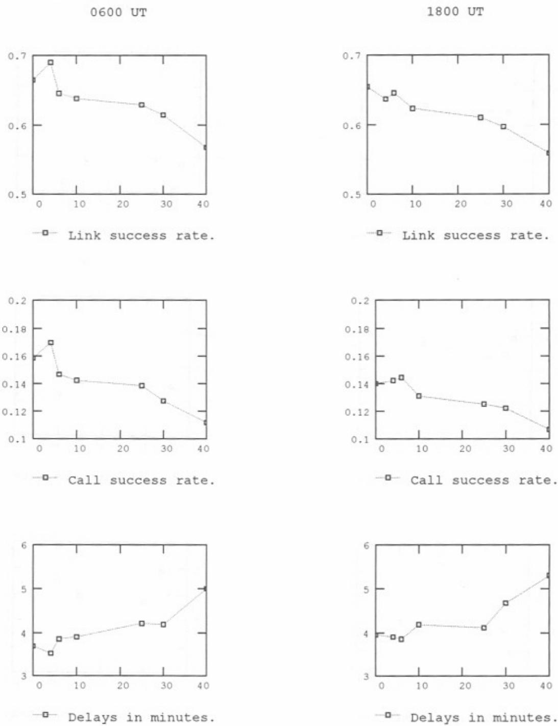
Figure E-10. Simulated network performance for 0600 and 1800 (UT) - 0, 4, 6, 10, 15, 30, and 40 scheduled sounds per hour - propagation condition 3 - 45 messages per hour.
