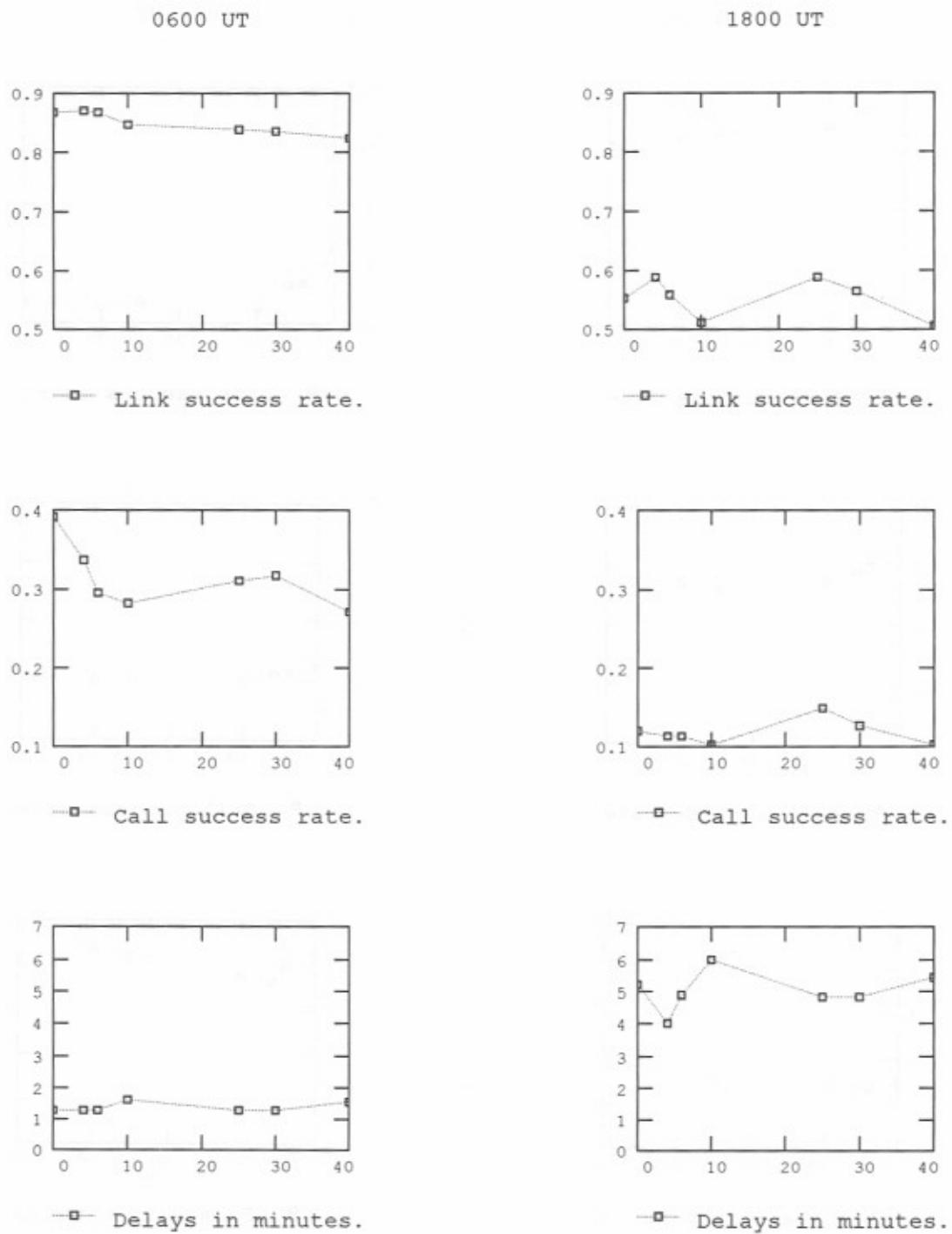
Figure E-12. Simulated network performance for 0600 and 1800 (UT) - 0, 4, 6, 10, 15, 30, and 40 scheduled sounds per hour - propagation condition 5 - 10 messages per hour.
