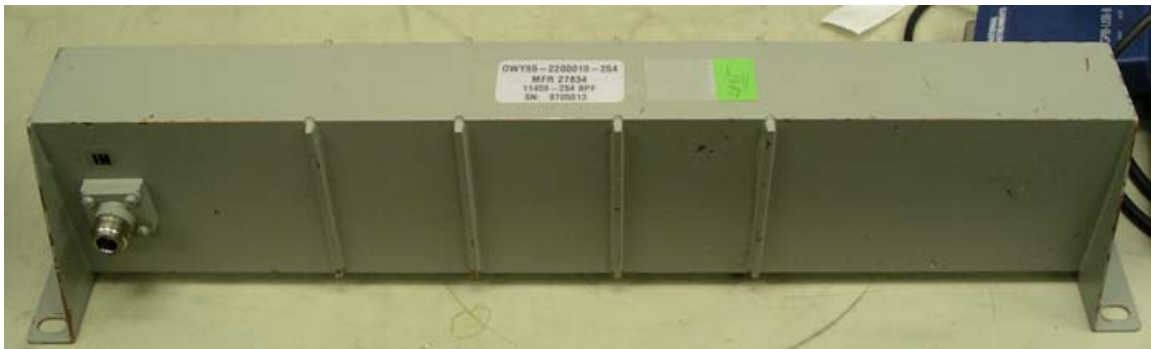
Figure 13. Weather radar receiver EMI bandpass filter.
