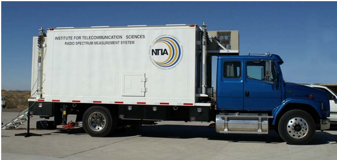
Figure 7. NTIA/ITS RSMS-4 vehicle. Major elements include an RF-shielded equipment enclosure, two telescoping masts, and an on-board power generator.
