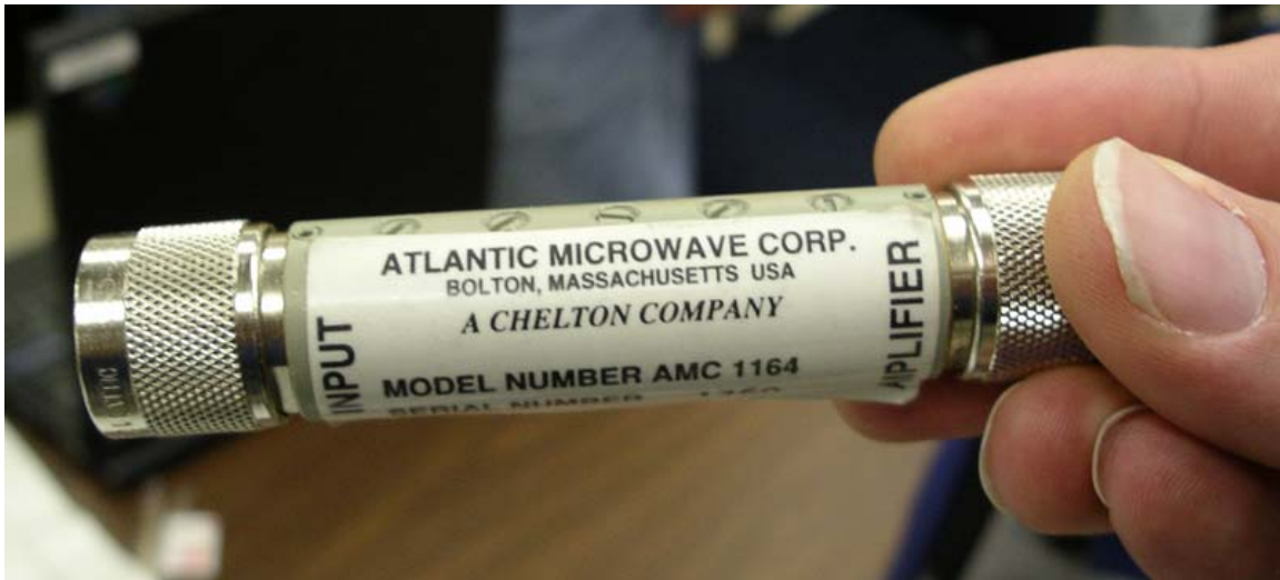
Figure 12. Weather radar receiver passive diode limiter.
