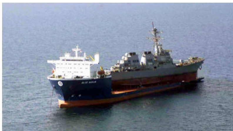
The Gulf of Aden, Oct. 31, 2000 — USS Cole is lifted by M/V Blue Marlin , a Norwegian dry dock vessel, off the coast of Aden, Yemen. Cole , damaged in an attack in Aden on Oct. 12, will be carried back to the United States by Blue Marlin over the next few weeks. U.S. Marine Corps photo by Sgt. M.C. Miller
