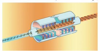
In a free electron laser, a relativistic beam of electrons is sent through an undulator, an array of dipole magnets with alternating north and south poles. The magnetic field of the undulator forces each bunch of electrons to oscillate back and forth, causing them to emit a laser-like beam of light. (Illustration by Flavio Robles, Creative Services Office)
