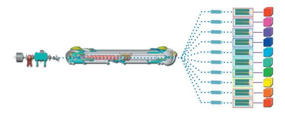
The next-generation light source facility envisioned for Berkeley Lab would use a superconducting linac to feed 10 or more free electron lasers, each tuned to the user's needs.
