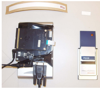
Figure 2.3: SkyeModule M8 reader with battery pack (left), and ACG Dual ISO CF Card reader (right) with the corresponding RFID labels.
