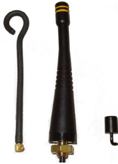
Figure 2.4: Standard Crossbow monopole antenna (left), Linxtechnologies PW monopole antenna (center), and embedded Linxtechnologies JJB antenna (right).
