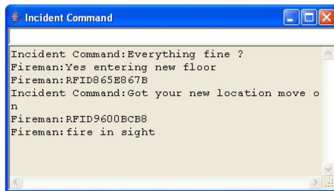
Figure 5.1: Text messaging communication GUI on the incident commander side - the one on the IPAQ looks identical.
