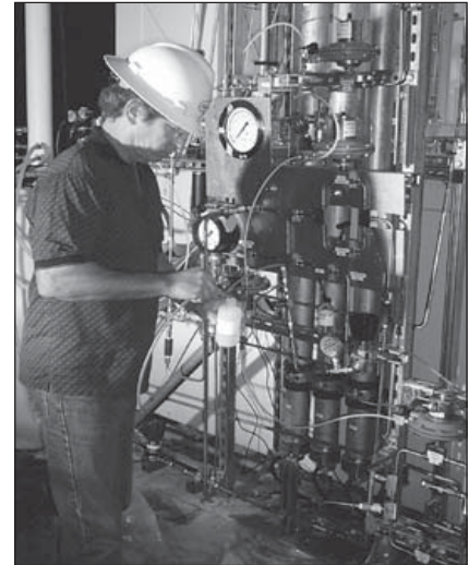
Surface laboratory at Frio uses pilot “U tube,” designed by Lawrence Berkeley National Laboratory, to extract hourly brine and gas samples for analysis
