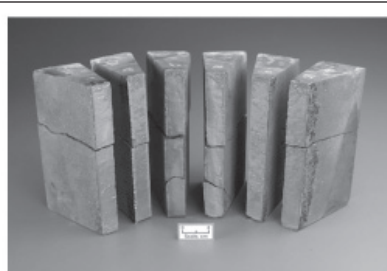
Conventional refractory after rotary slag testing.
