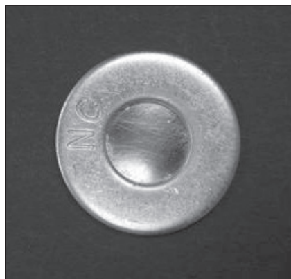
A mounted 3/4-inch diameter Pd-Cu alloy membrane for hydrogen separation
