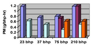
Exhaust gas composition was measured with an Enerac Model 300 portable emission analyzer. PM was measured by weighing the accumulation of particulate on a quartz filter with no dilution tunnel. Formal fuel performance tests were not conducted, but the operator stated there was no noticeable change in consumption when the continuous water injection system was applied.
