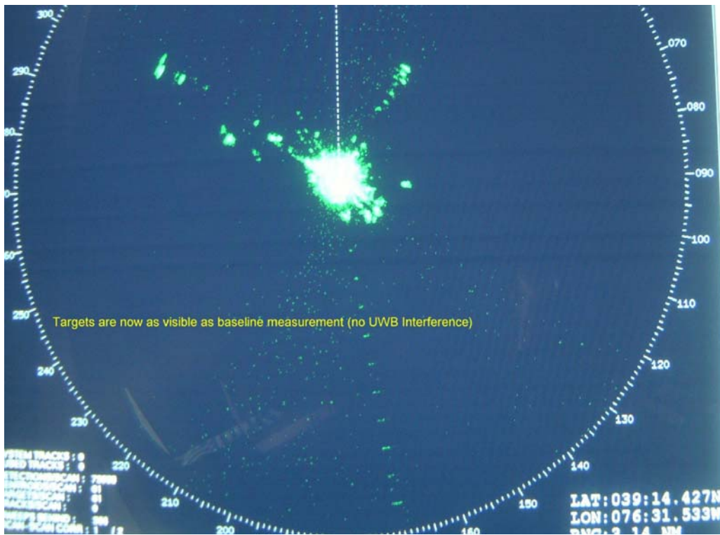
Figure 61. Radar A PPI display with 10-MHz prf UWB signal at -116 dBm/MHz (RMS detection).
