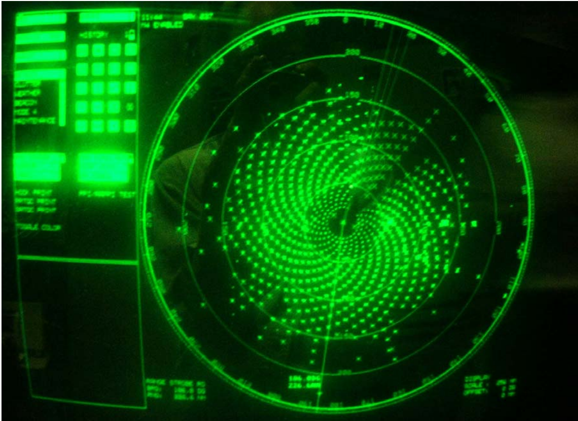
Figure 17. Sector-wedge distribution of desired targets on a PPI display during testing on a long-range air search radar. Targets are shown as “+” signs, and are generated at the radar RF stage.
