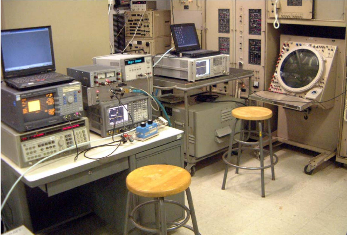
Figure 14. Typical arrangement of NTIA interference and target generators at an air search radar station. The NTIA equipment is spread across the table in the foreground and the cart in the background, with the radar PPI display at right.
