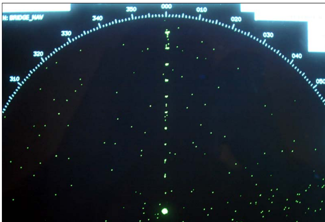
Figure 48. 1- \mu s pulsed interference at 7.5% duty cycle and I/N = +12 dB.
