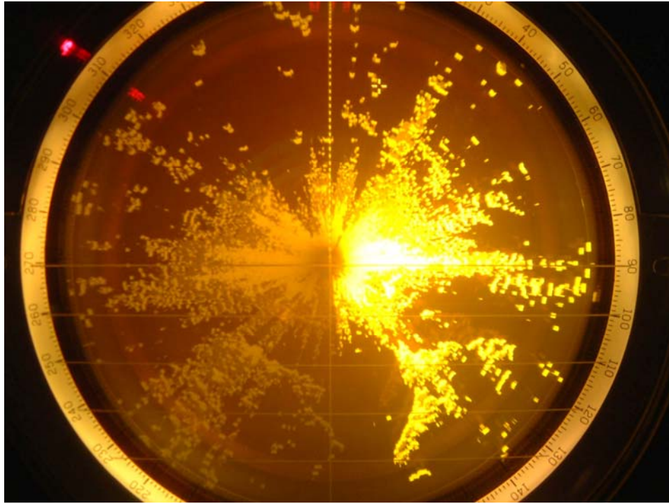
Figure 4. An example of clutter on a 9-GHz maritime radionavigation radar plan position indicator (PPI) display. The clutter includes local buildings, terrain, and vegetation. No intentional interference or test targets are present on this display.
