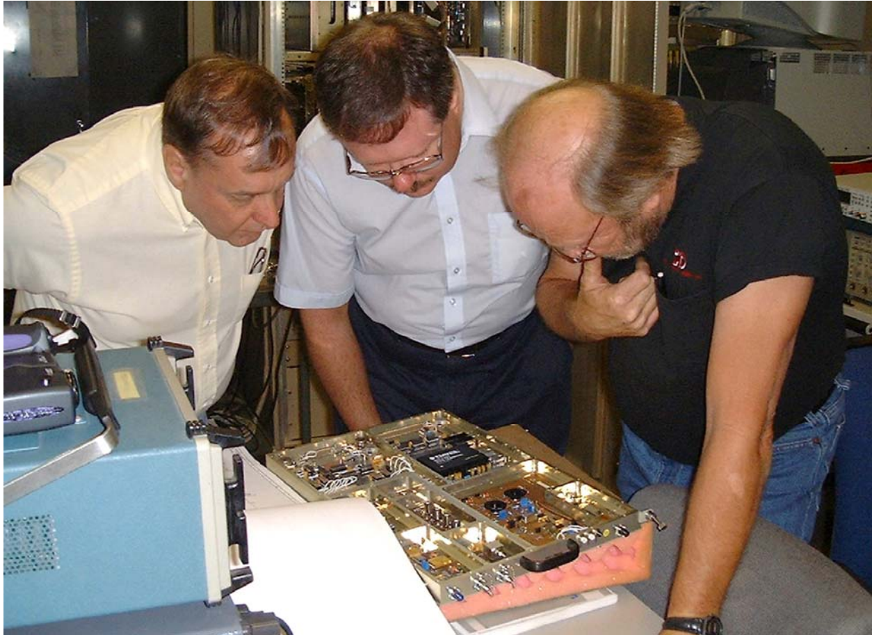
Figure 11. NTIA and FAA engineers determining the locations on a radar IF-stage circuit card where the I/N level could be monitored.
