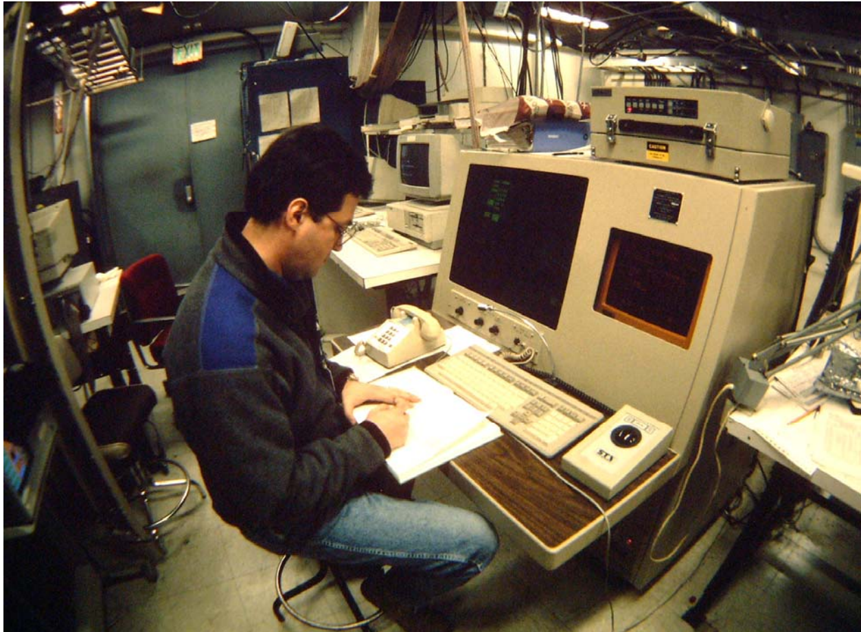
Figure 9. Typical conditions inside an air-search radar station, showing the main console for display and control.
