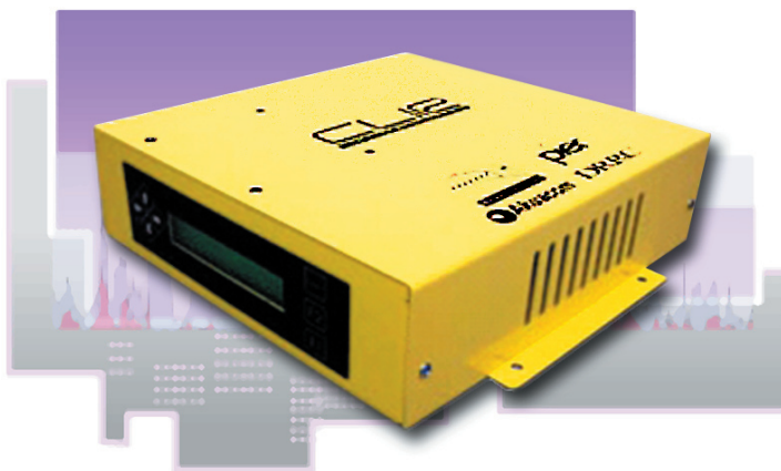
The CLIR box, a Client Logic Integrated Relay, is an analog-to-digital signal processor developed by the Demand Response Research Center, which allows building systems to receive automated demand-response signals inexpensively.
