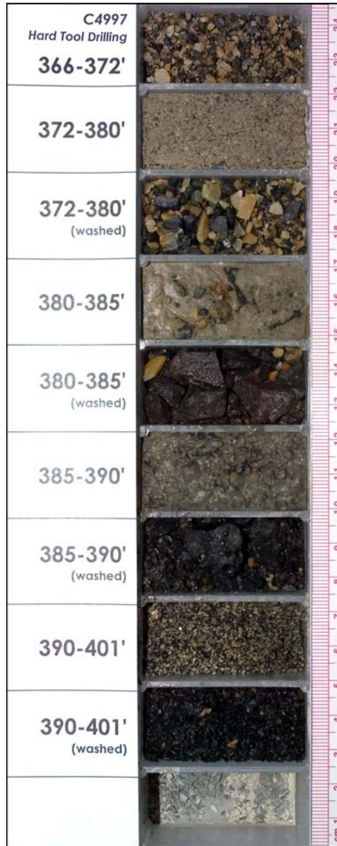
Figure 3.3. Example of Drill Cuttings from the Ringold Formation Unit A from the Bottom of the C4997 Entry Borehole. All the samples in this tray were pulverized during hard-tool drilling and therefore are not representative of the true grain-size distribution. Each sample interval (except 366–372 ft) is shown twice, once before rinsing away of mud generated during drilling and again after rinsing away of fines (washed). Relatively low basalt content and rusty iron-stained color (characteristics of Ringold Unit A), both in the washed and unwashed samples, are visible between 366- to 380-ft depths. The basalt contact at 383 ft is apparent based on the sudden increase in blocky, angular basalt fragments in the 380- to 385-ft (washed) sample.
