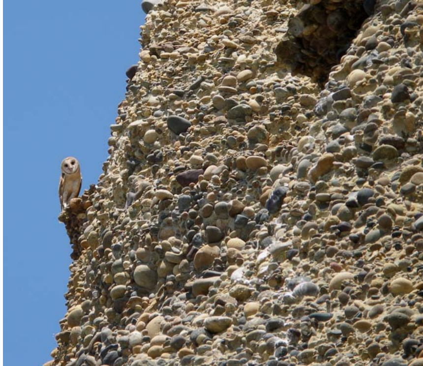
Figure 3.4. An Analogue for Ringold Formation Unit A Exposed Along the White Bluffs, 15 Miles East of the Waste Treatment Plant. Note bimodal texture of clast-supported pebble-cobble conglomerate within matrix of well-sorted, fine to medium sand. Also note pervasive rusty colored, iron-oxide stain. Gravel clasts, composed of only 10–20% basalt, are well-rounded and polished, characteristic of a fluvial deposit.
