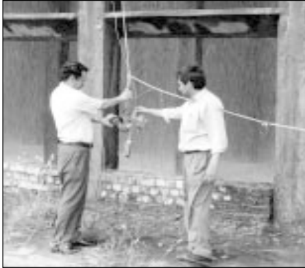
Engineers measuring wet-bulb temperature of air at the cooling tower inlet
