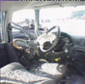
Driver area overview Toe pan intrusion 18.5"
