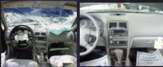
No driver toepan intrusion!
