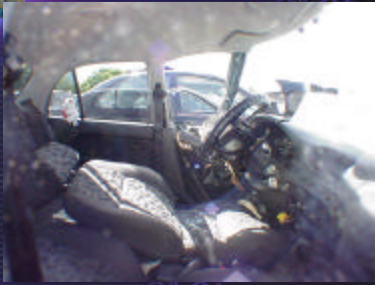
Left instrument panel intrusion 15"
