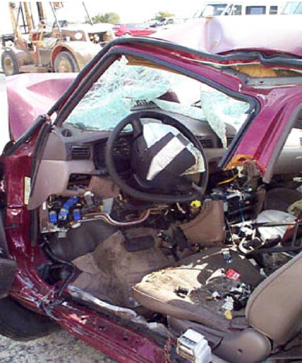
Left: dash (32), toe pan (86), steering assembly (31), A-pillar, floor pan (15) intrusion.
