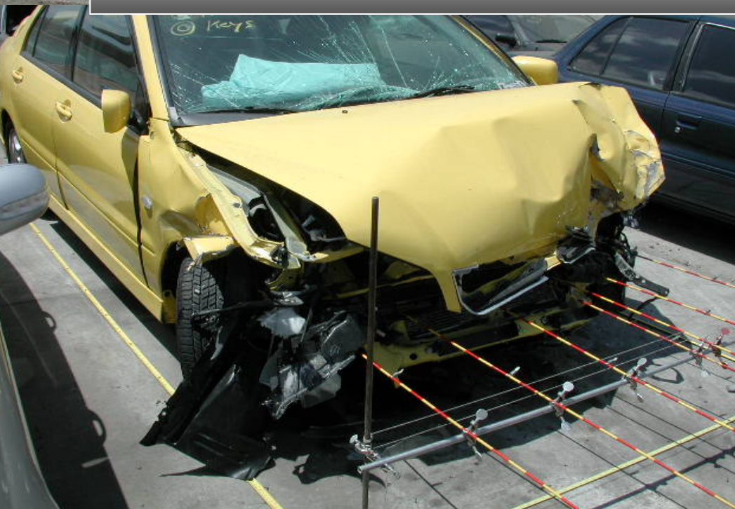
2002 Mitsubishi Lancer / 54 cm Max. crush / 34 mph DV / 12:00 PDOF
