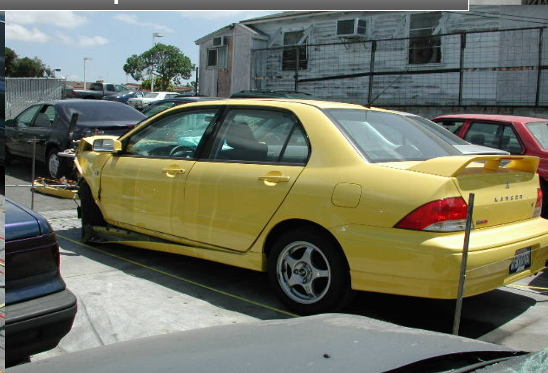
2002 Mitsubishi Lancer / 54 cm Max. crush / 34 mph DV / 12:00 PDOF
