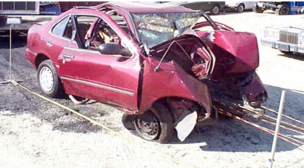
1996 Nissan Sentra / Max. crush = 135 cm / 12:00 PDOF / 66mph dV (stvz 45mph)
