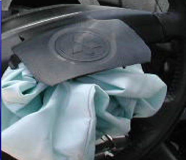
Contact: lower dash/bolster, belt, air bag, steering assembly
