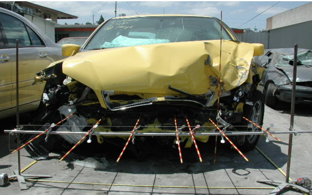
2002 Mitsubishi Lancer / 54 cm Max. crush / 34 mph DV / 12:00 PDOF
