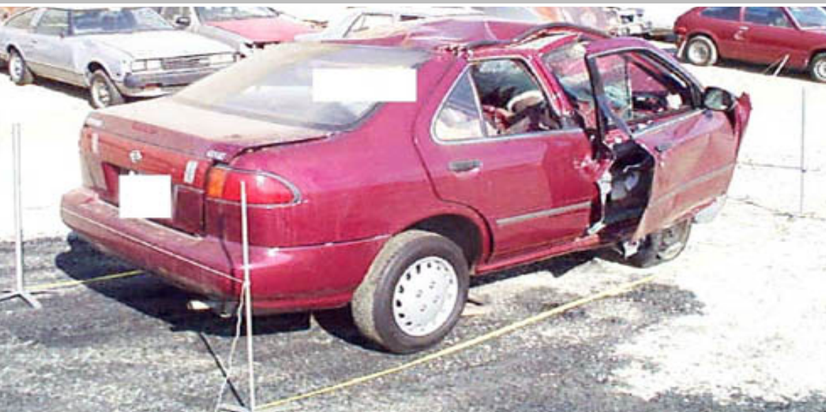
1996 Nissan Sentra / Max. crush = 135 cm / 12:00 PDOF / 66mph dV (stvz 45mph)
