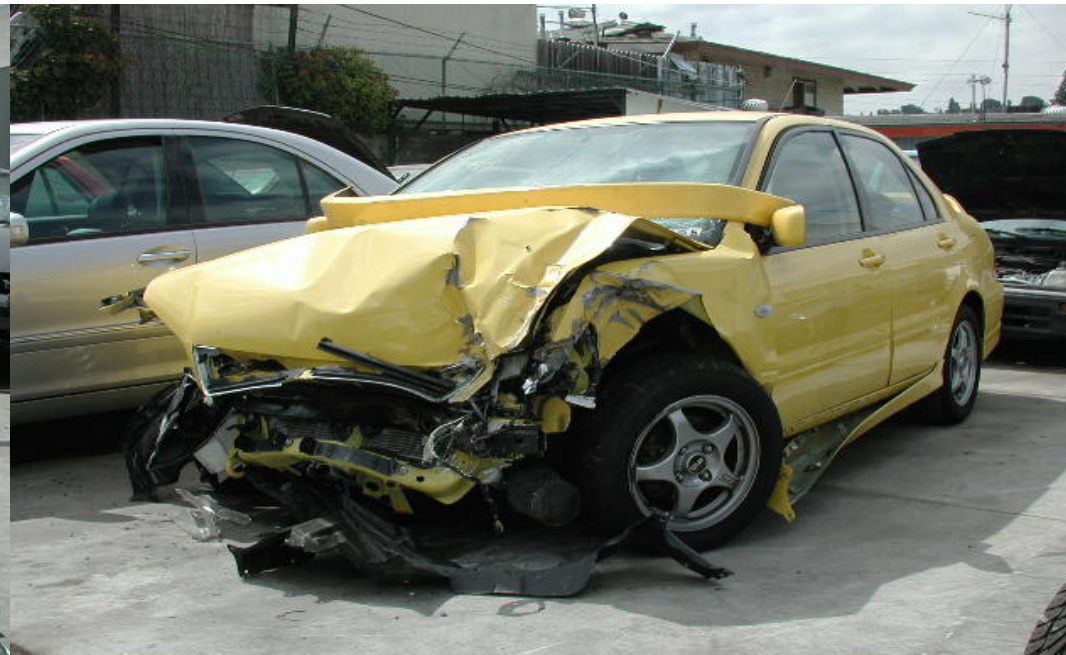
2002 Mitsubishi Lancer / 54 cm Max. crush / 34 mph DV / 12:00 PDOF
