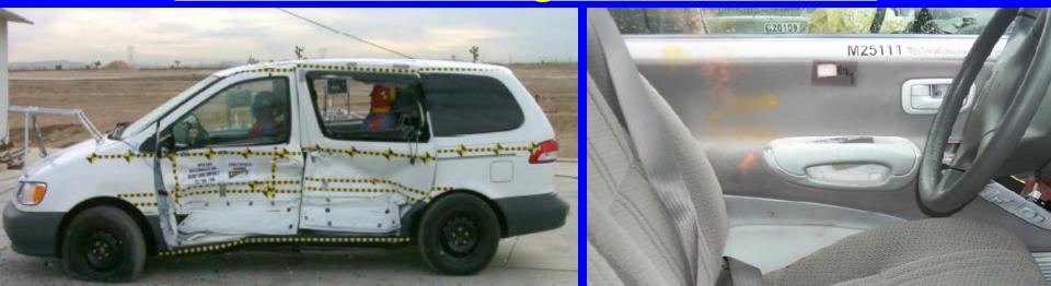
2001 Toyota Sienna, Weight = 2029 kg, Door crush = 29.7 cm Driver TTI = 69, pelvic g = 94, No side airbag
