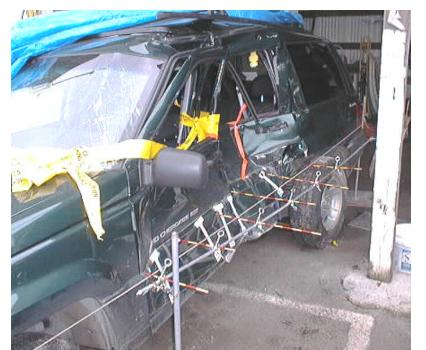
Door Extrication - low profile  $\checkmark$ Delta V = 15 mph PDOF = -80
