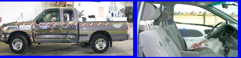
2002 Toyota Tundra, Weight = 2229 kg, Door crush = 29.8 cm Driver TTI = 22, pelvic g =27, No side airbag
