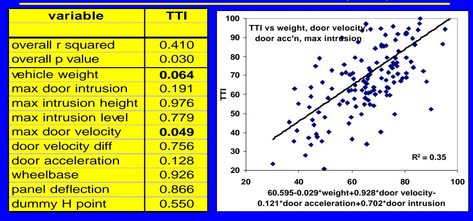
Vehicle weight and max door velocity correlate to TTI
