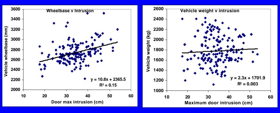
Door intrusion, weak correlation to wheelbase ( $r^2 = 0.15$ ) Door intrusion, none to vehicle weight ( $r^2 = 0.003$ , NS)
