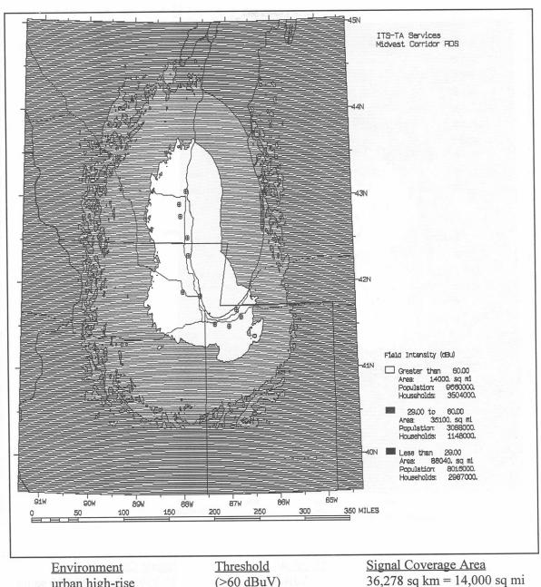
Figure 4. Composite FM station RBDS subcarrier coverage for Corridor 2, Midwest.
