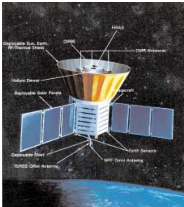
Figure 1. Artist's rendering of COBE satellite with callout of instruments and components.
