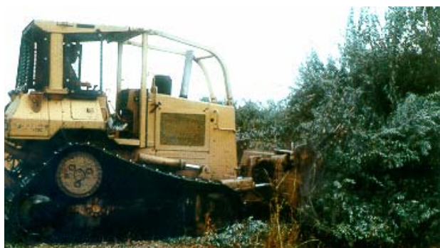
Dozing of Russian-olives near Richland, WA. Severed top growth was piled and burned. Soil disturbance was considerable.
