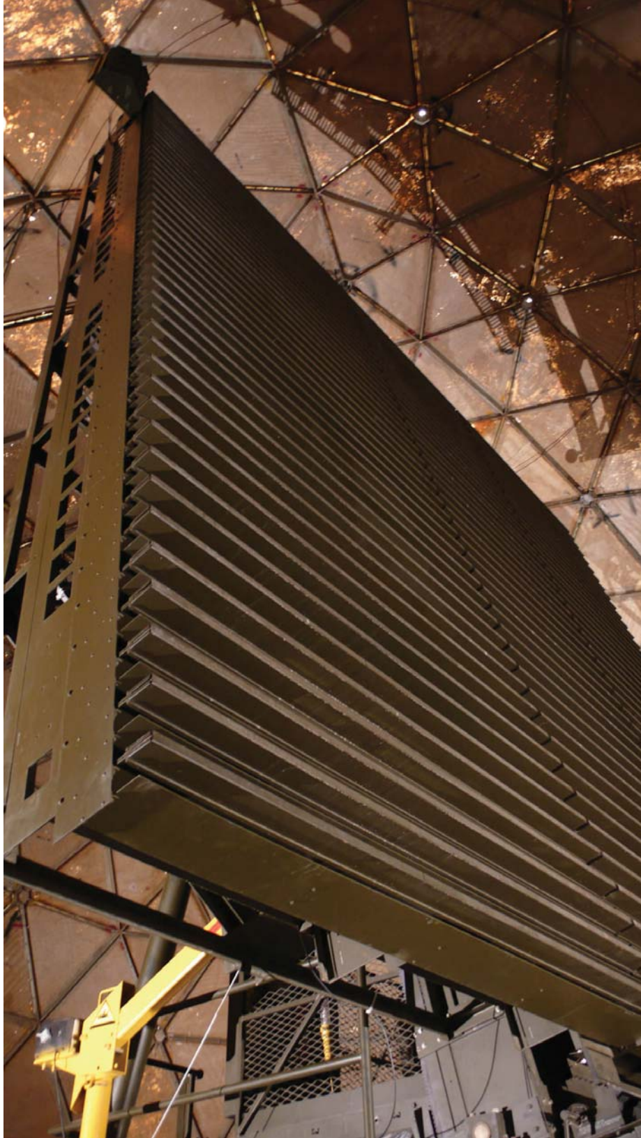
The antenna of an air search radar during interference testing (photograph by F.H. Sanders).
