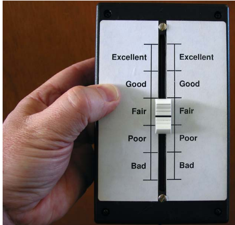
Figure 1. SSCQE-HRR subjective rating device used for HDTV experiment (photograph by S. Wolf).
