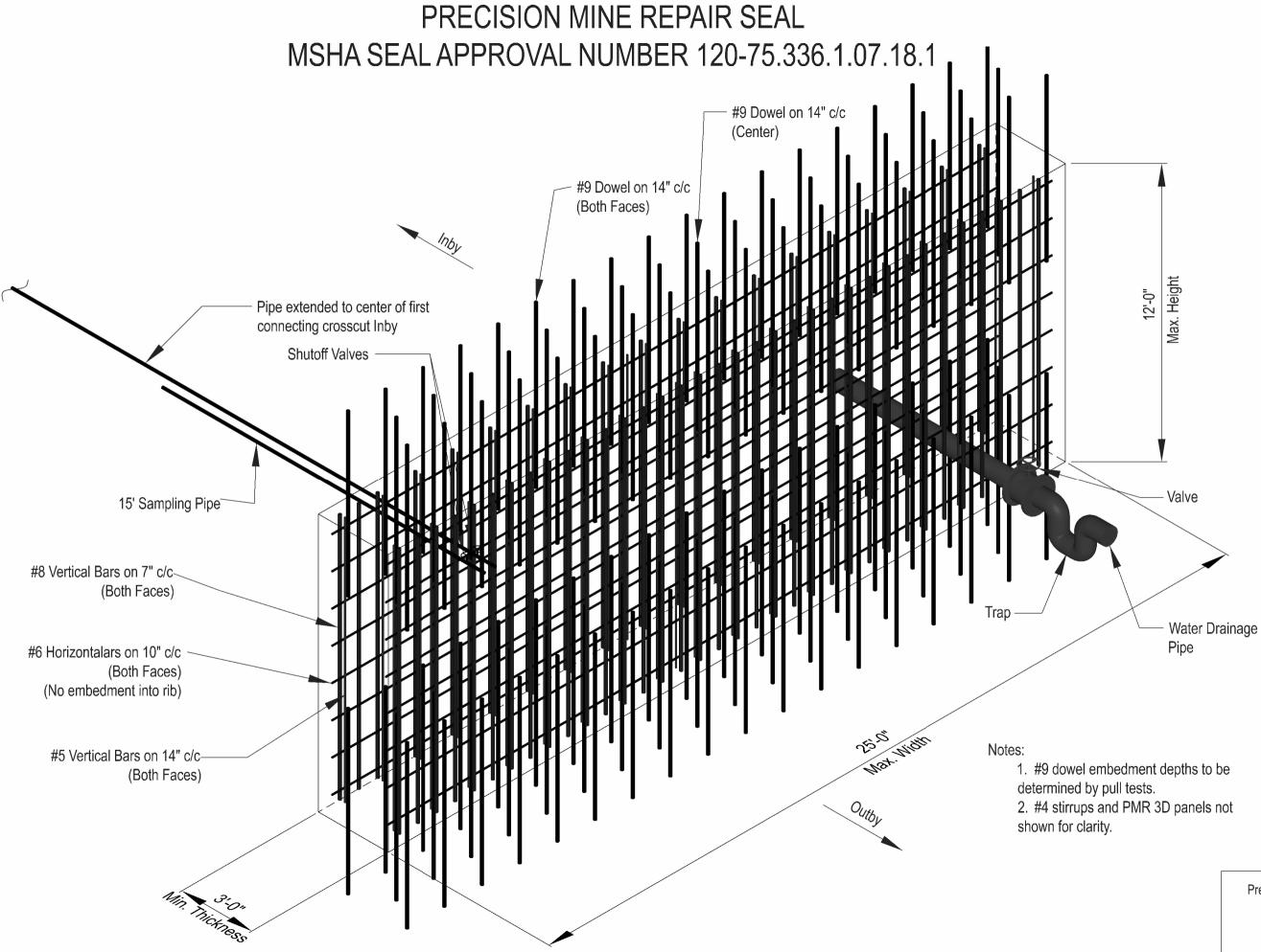
Precision Mine Repair 120 PSI Isometric View Figure #1
