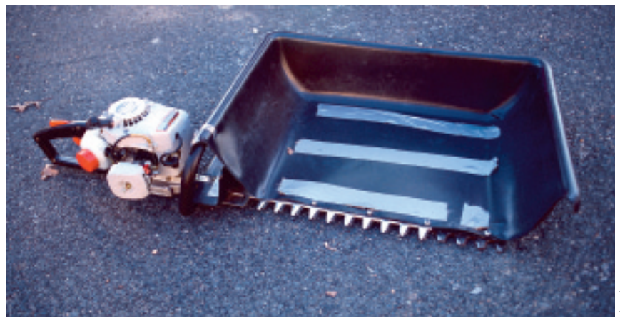
Figure 1 • A modified gas powered hedge trimmer ready to harvest native plant seeds.
