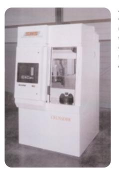
A new high-precision vertical lathe which incorporates the new thermal-error compensation technology, first delivered to customers in 1998.
