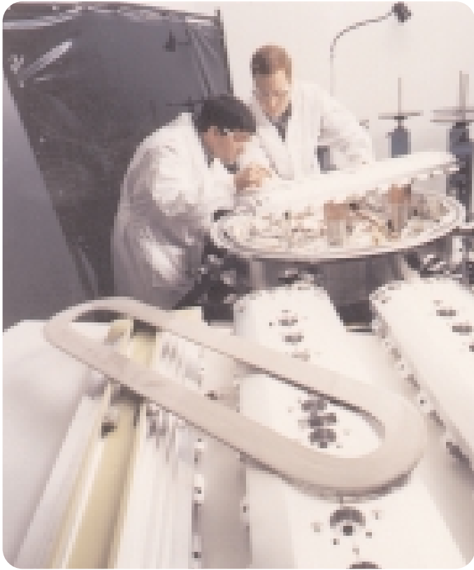
Placing 1000 horsepower HTS motor coils into a cryogenic cooling system.
