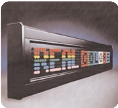
The Real Color Display™, a moving sign which is capable of displaying the full range of colors, made possible by the use of blue LEDs.
