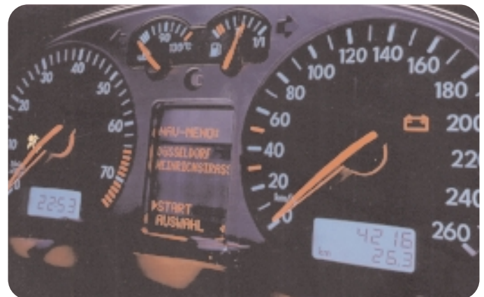
Cree's LED chips are used by Siemens A.G. for back lighting for this dashboard.
