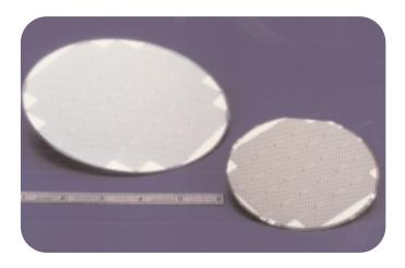
Vitesse's ability to fabricate chip's on 6" wafers in it's new plant, (instead of 4" wafers) more than doubles the number of intergrated circuits that can be fabricated on each wafer and increases the efficiency of production.
