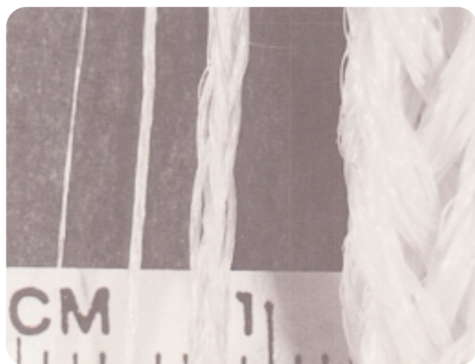
Collagen fiber and braided structures from collagen fiber: (a) single collagen fiber, (b) 8-ply collagen fiber braid, (c) 64-ply collagen fiber braid, (d) 512-ply collagen fiber braid.
