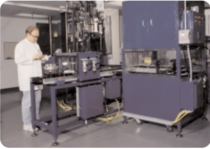
An automated gelcasting machine capable of forming 10,000 ceramic turbine wheels per year.
