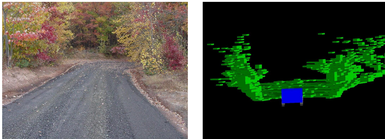
Figure 1. (left): Digital camera image of road and trees; (right) the same scene as viewed by Demo III real-time LADAR. Where does the technology fall short? The vehicle is effectively myopic. Current LADAR is low resolution (75 mm to 150 mm accuracy) and short range (<40 m returns from horizontal surfaces). Current LADAR does not penetrate dust and smoke. Planning is not optimized for road following.
