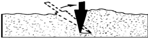
1. Insert dibble at angle shown and push forward to vertical.
