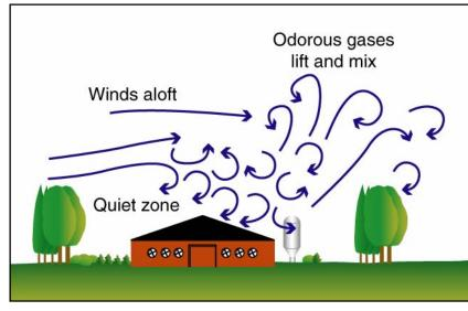
height, beyond the windbreak. Backpressure created by the blocking effect of the tree row also creates a small quiet zone upwind of the tree line that is equal to 2 to 3 times the height of the trees.
