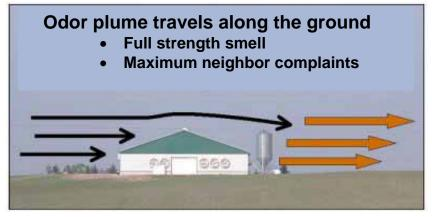
Figure 2 Without windbreaks and wind management, the odor plumes are picked up by passing air masses and travel near the ground with little or no dilution or filtration.
