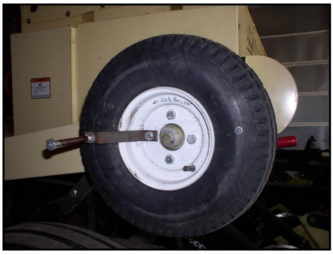
Figure 4. Floating drive wheel with drive handle for calibration, and number of and direction of rotation for drill calibration.
