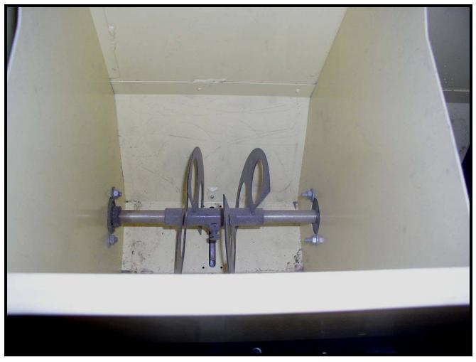
Figure 6. View of inside of fluffy box showing agitator and picker wheel.
