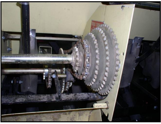
Figure 7. Derailleur controls for fluffy seed box. Moving the chain to the left increases seed output and moving the chain to the right decreases seed output.
