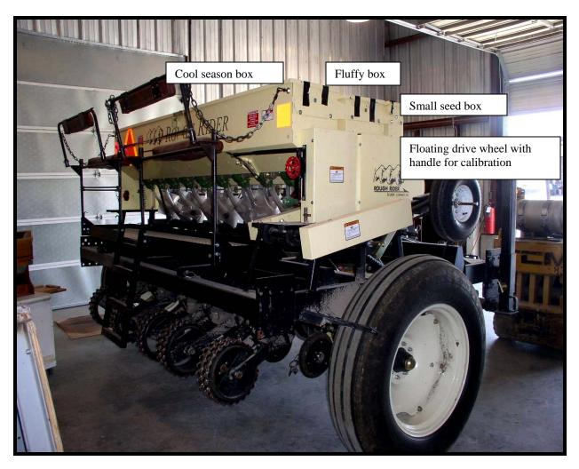
Figure 2. Truax Roughrider seed drill showing location of seed boxes and floating drive wheel with handle for calibration,
