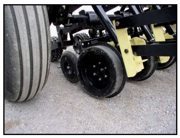
Figure 1. Close-up view of drill seeding unit.
